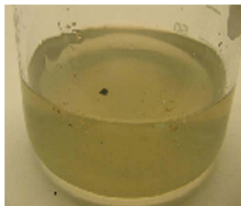
Figure 4 Black particle in HFIP-Chloroform solution of chips. [Color figure can be viewed in the online issue, which is available at wileyonlinelibrary.com.]
